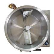
Scrapers at tank bottom & side for complete coverage
